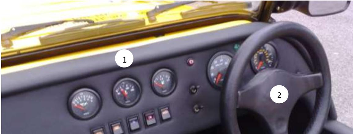
3. Remove dash retaining bolts (3mm allen key).
